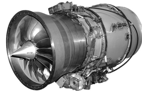
Williams International FJ44-3A engine(Sutliff, D. L. et al., 2013)
