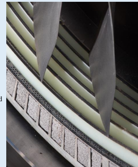
OTR acoustic casing treatment (Bozak, R. F. et al., 2018)
