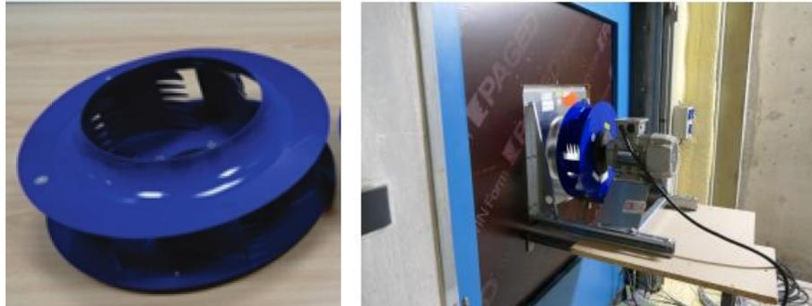
**Excerpt from Deliverable 5.1:** Numerical and experimental research were carried out on the influence of Leading-Edge and Trailing-Edge serrations on aerodynamic and noise performance of a low speed cooling fan industrial application
