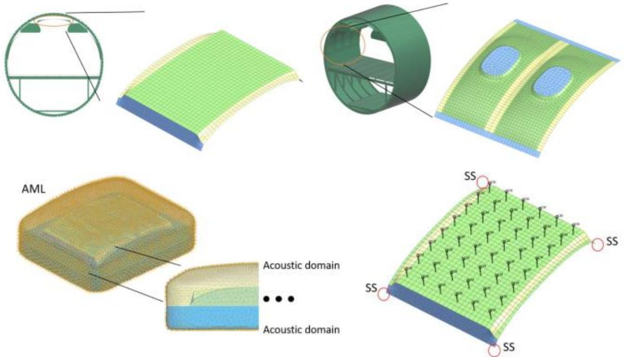
**Excerpt from Deliverable 5.4:** Numerical research was conducted to evaluate the performance of the addition of tuned vibrations absorbers (TVAs) on the fuselage dominant noise transmission paths, in order to improve the noise radiated into the aircraft's cabin
