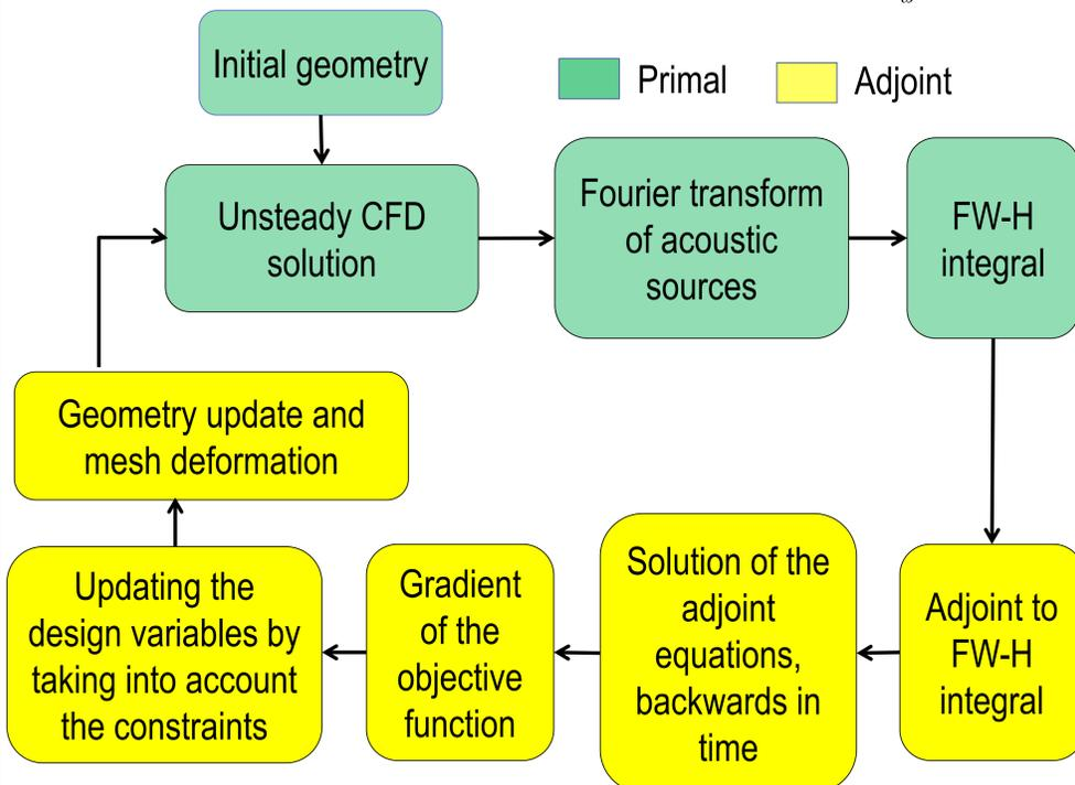
Fig. 1: Work flow of the aeroacoustic shape optimization
