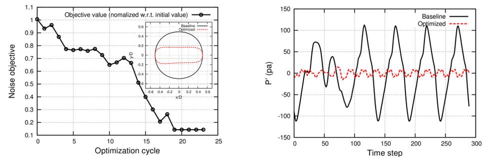
Fig. 3: Convergence of the objective function and geometry after reaching the minimum volume constraint (left). Reduction of fluctuations in the optimized geometry (right).
