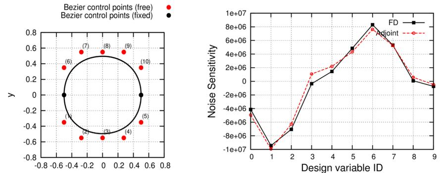
Fig. 2: Parameterization using Bezier curve (left) Good agreement between the adjoint and finite difference gradients (right).
