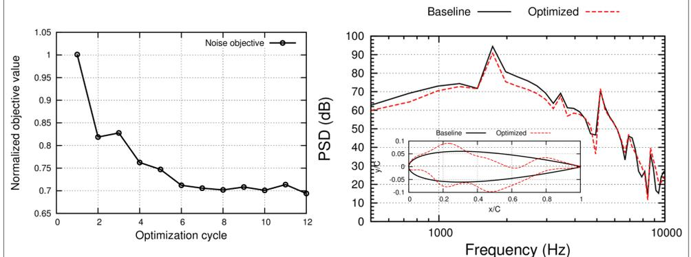
Fig. 5: Convergence of the objective function (left). Comparison of the PSD plot of the sound pressure between the baseline and optimized geometry (right).
